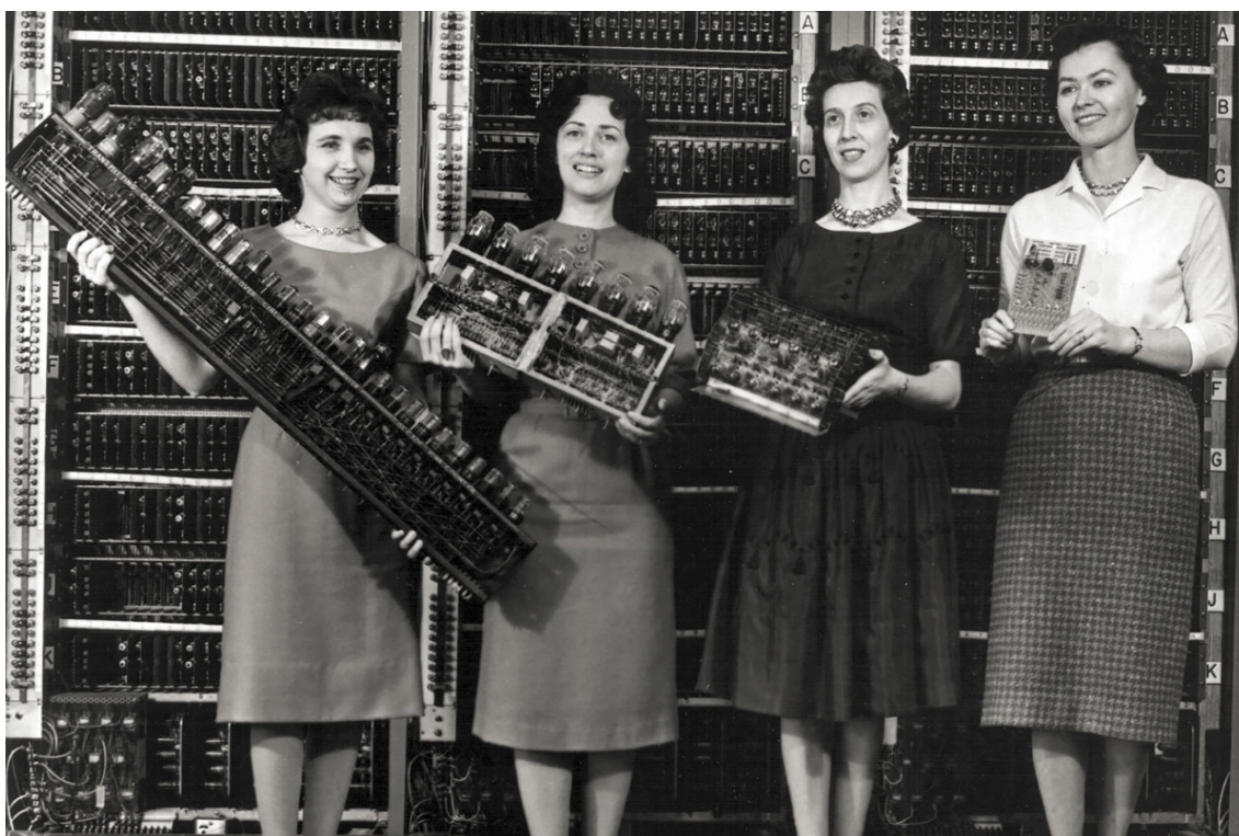
Figure 7: Patsy Simmers, holding ENIAC board; Gail Taylor, holding EDVAC board; Milly Beck, holding ORDVAC board; and Norma Stec, holding BRLESC-I board. U.S. Army/ARL Technical Library Archives
